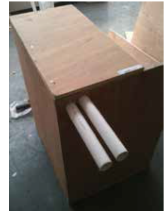
Dip and vent tubes exit through side of hut to exterior Hydrogen gas vet tube turns up at end, cold air tube is a straight exit. Both tubes have mesh covering to prevent insects from entering
